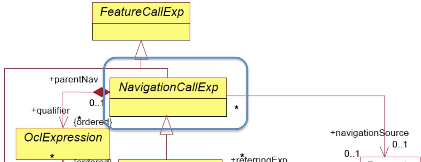
A ***NavigationCallExp*** is a reference to an *AssociationEnd* in an *ECore* model. It is used to determine objects linked to a target object by an association.
