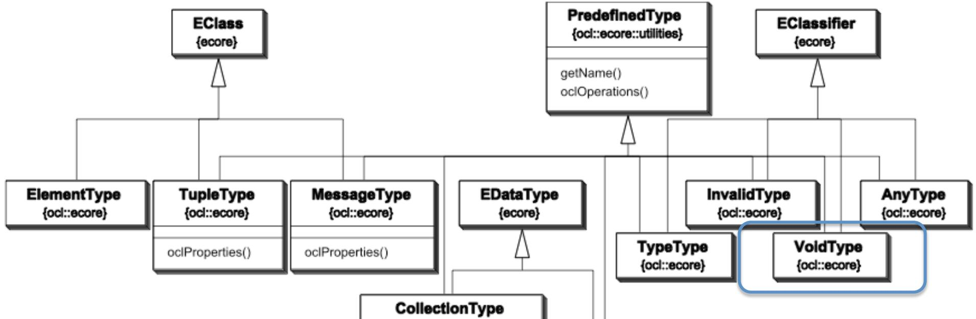
*VoidType* conforms to all types. The only instance of *VoidType* is “*oclVoid*”
