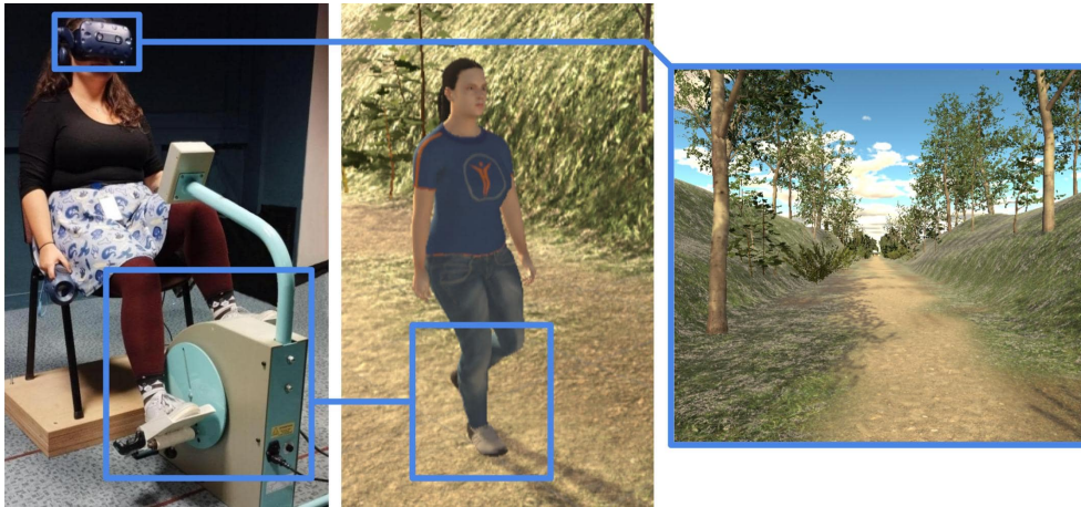
Figure 3: We introduce assisted motion to walking-by-cycling using a motorized bike (left). The user embodies an avatar which is viewed in first-person perspective (right). The bike drives the user's legs in a cycling motion, which makes the avatar walk in synchrony (middle) without requiring effort from the user.
