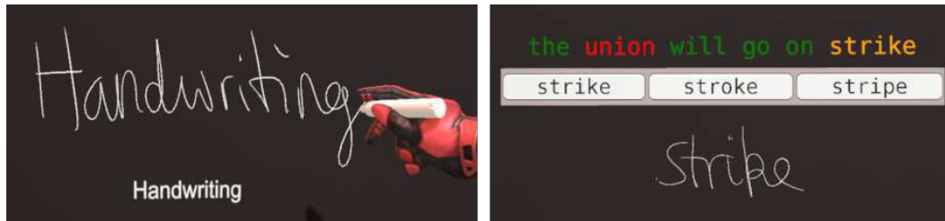
Figure 5: The user can write words by hand on a board in the virtual environment. Handwriting recognition technology converts the handwritten word into usable text data (left). During the user study, participants are presented with phrases they have to write one word at a time (right). The yellow word is the selected word. Green words are correctly recognized and red words are not. Users are presented with multiple recognition results they can choose from.
