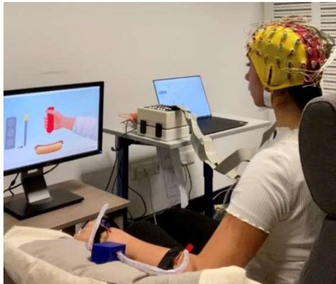
Figure 24: The GRASP-IT approach for BCI and post-stroke rehabilitation: three vibrotactile motors are located on the hand and the forearm. Their activation rotation frequencies and duration are synchronized and analogous to the visual feedback corresponding to four different levels of a grasping movement.
