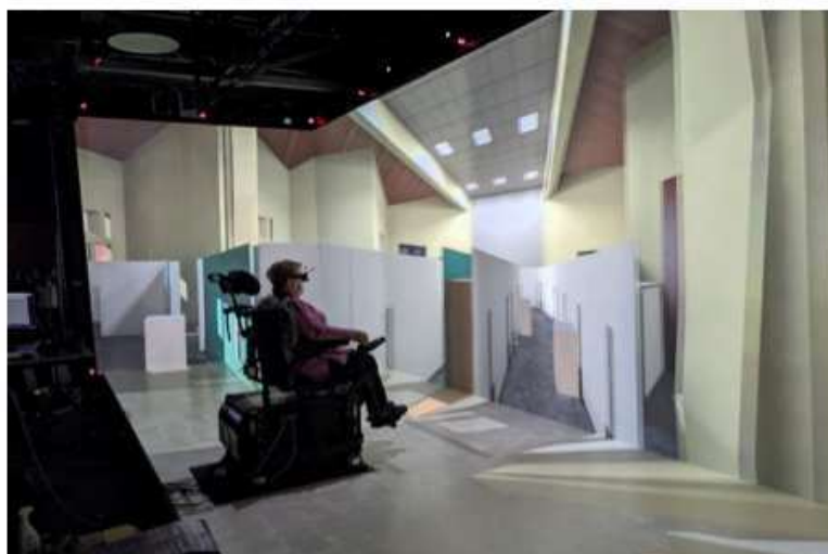
Figure 4: The wheelchair simulator tested by a volunteer in immersive conditions.
