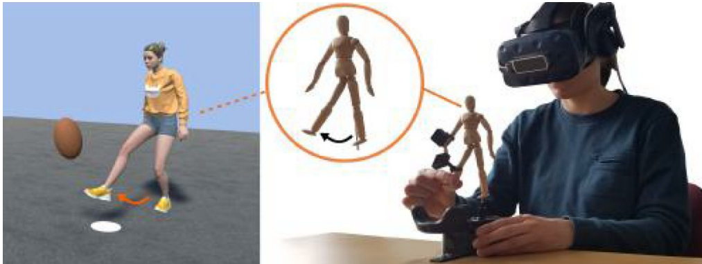
Figure 17: We propose to use a tangible prop to control a human-like avatar during seated virtual experiences. By manipulating the prop, users perform kinematics similar to those of the avatar and experience physical interactions with it. We show that such controllers can enhance the sense of presence and embodiment compared to traditional gamepad controllers.
