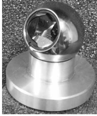
Figure 4.2: CCR target used with the laser tracker.
