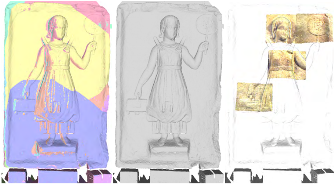
Figure 6.7: Registration of the ten meshes. (a) One color per mesh. (b) All meshes in grey. (c) Color image from multispectral data projected on the 3D model.
