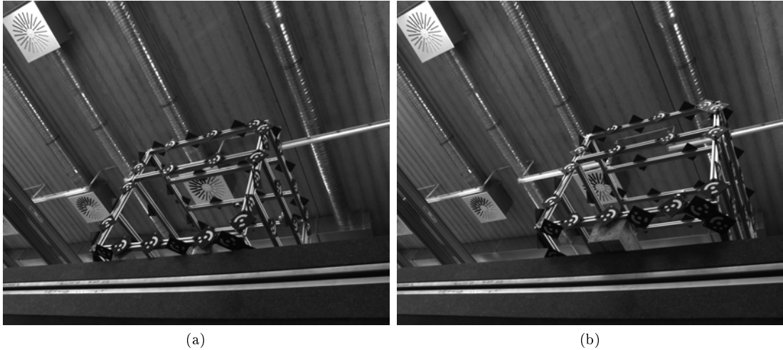
Figure 4.9: Target frame on the marble table seen from a bottom tracking camera. (a) representative of the badly tracked positions M1, M2 and M5. (b) representative of better tracked positions M3 and M4.
