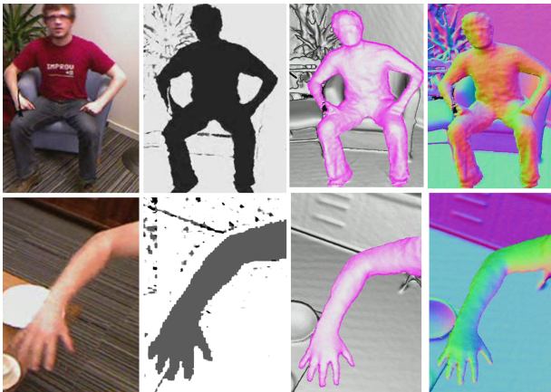
Figure 15: Moving user is segmented and reconstructed, independent of background. Left to right: 1) Live RGB. 2) ICP outliers (for initial segmentation prediction). 3) final composited scene showing foreground shaded differently to background. 4) Composited normal maps.
