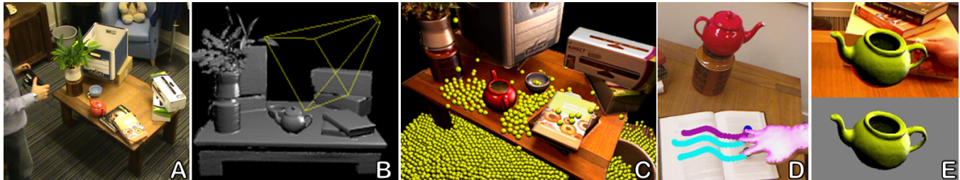
Figure 1: KinectFusion enables real-time detailed 3D reconstructions of indoor scenes using only the depth data from a standard Kinect camera. A) user points Kinect at coffee table scene. B) Phong shaded reconstructed 3D model (the wireframe frustum shows current tracked 3D pose of Kinect). C) 3D model texture mapped using Kinect RGB data with real-time particles simulated on the 3D model as reconstruction occurs. D) Multi-touch interactions performed on any reconstructed surface. E) Real-time segmentation and 3D tracking of a physical object.
