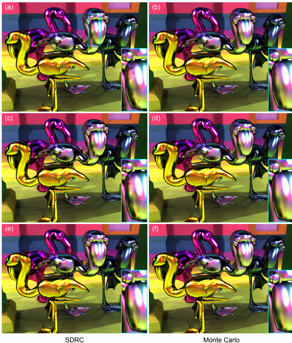
Figure 2.7 – Rendering time scalability. The images were rendered at a resolution of 1024 \times 768 . Images on the left shows rendering quality of the SDRC for the value of N set to N = 64, 128 and 256 . Images on the right were rendered using the MC in approximately the same time for the indirect term computation on glossy surfaces, as the top images, 76, 153 and 269 seconds, respectively.
