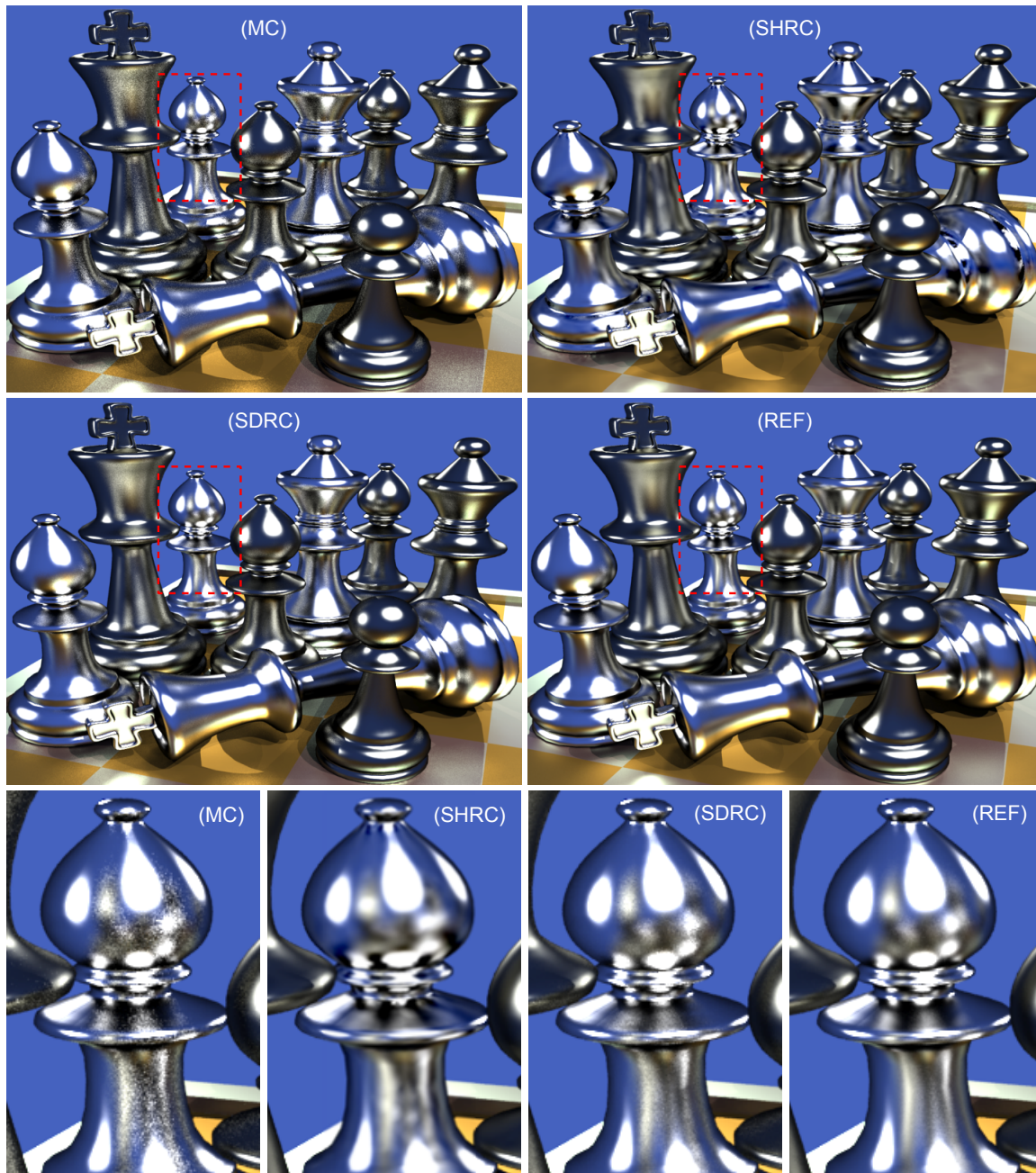
Figure 2.6 – Renderings of the chess scene. Images were rendered at a resolution of 1024 \times 768 in approximately the same time, 468 seconds. The indirect term computation on glossy surfaces took 365 seconds. Note the sharper glossy reflection of black pieces on the white chess piece in the details. Chess pieces courtesy of Toshiya Hachisuka.
