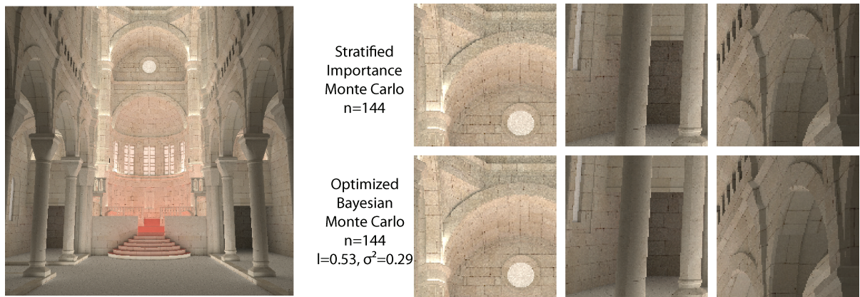
Figure 9: Optimal BMC rendering of the Sibenik Cathedral (Indirect only). n = 144 , \bar{l} = 0.53 , \bar{\sigma}^2 = 0.29 . Locally, OBMC performance depends on how close are the global values of \bar{l} and \bar{\sigma}^2 to the local optimal values. Note that O-BMC never performs worse than SI-MC, hence the global quality of the rendering is improved. The overall reduction of the RMSE value is 11%. The reduction of the RMSE value for each of the detail view is respectively 8%, 22% and 16%.
