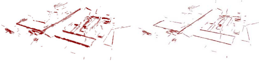
Figure 5: 3D view on matched line segments (left) and fitted line segments (right).
