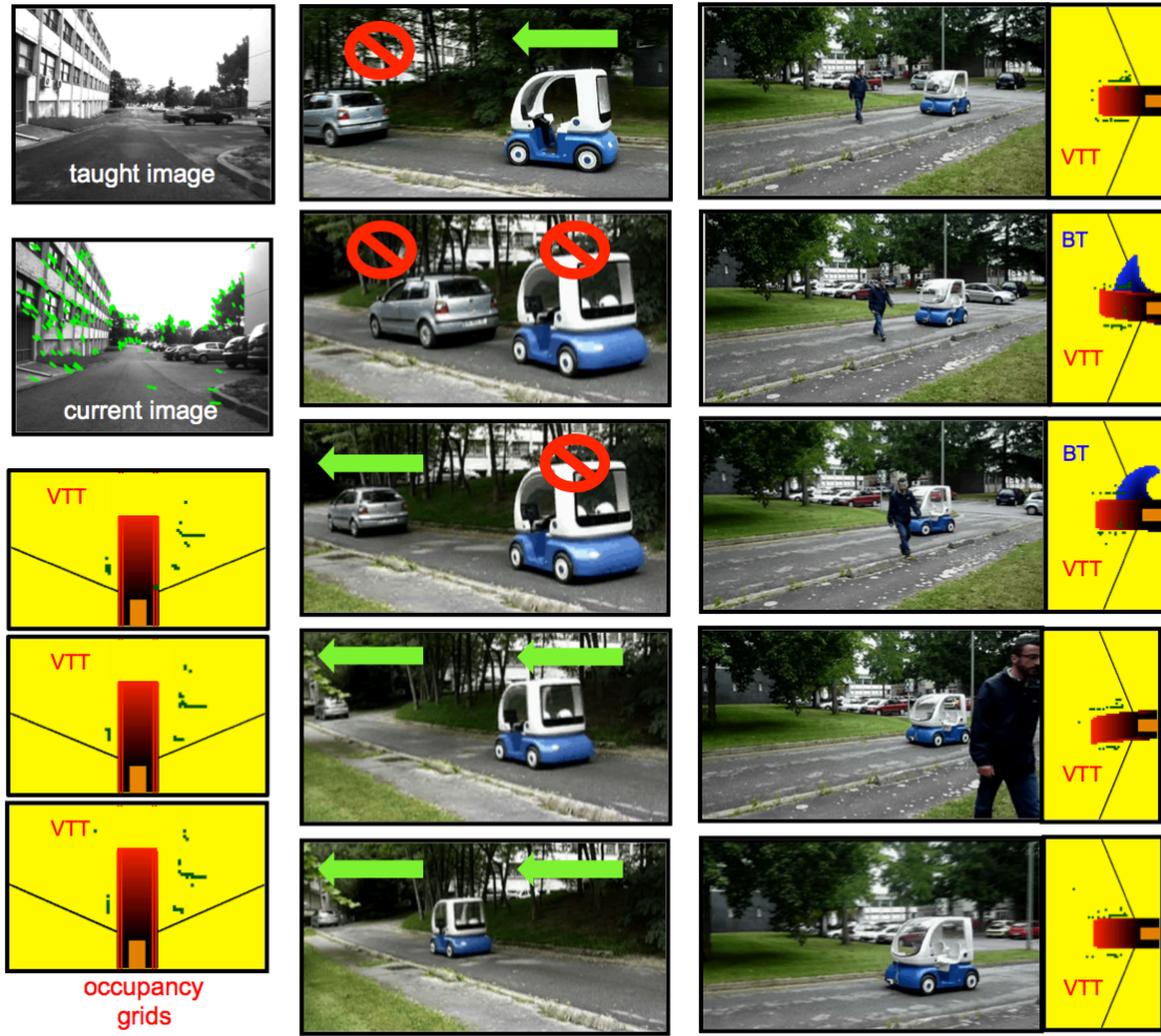
Figure 12: Validation with: irrelevant obstacles (left), traffic (center) and a moving pedestrian (right). The visual task tentacle and best tentacle (when different) are respectively indicated as VTT and BT in the occupancy grids.
